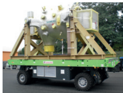
New from TII Group and Scheuerle is the battery powered SPMT Light with a capacity of 86 tons.
