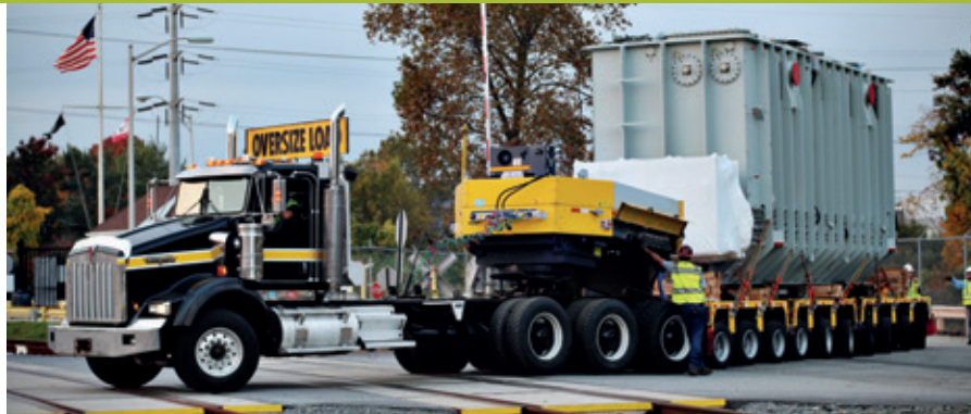
The latest product included in the Cometto product range is the MGSL modular axle lines that have a capacity of 50 to 5,000 tons.
