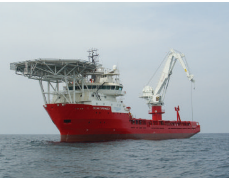
Knuckle boom crane using Python Compac 35 rope, which is 50 mm diameter, 2,070 m long
