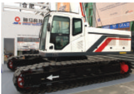
Hefei Smarter Technology's 50 tonne capacity SMQ500D telescopic crawler crane is one of eight models offered from 25 to 100 tonnes
