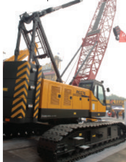
70 tonne capacity Rongsheng lattice boom crawler crane. Main boom is up to 57 m
