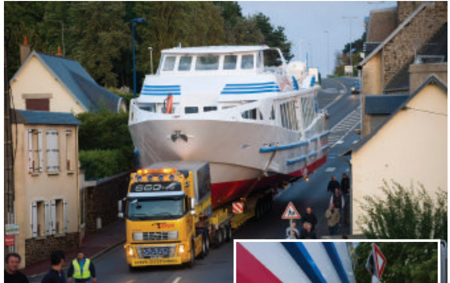
The 55 tonne boat was transported on a Nicolas MDEL platform trailer, with 3 + 5 axle lines and flat bed deck
