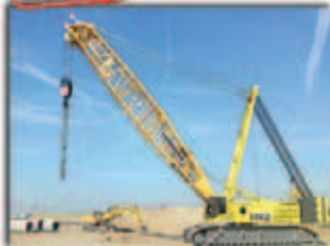
300 t Liebherr, LR 1300, Y. 2009 with derrick and luffing jib
