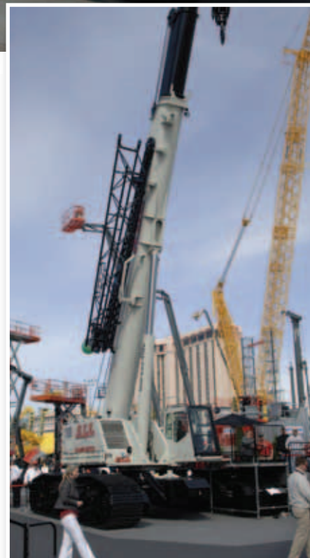
The new 110 ton (100 tonne) capacity TCC-1100 Link-Belt telescopic crawler seen for the first time at ConExpo
