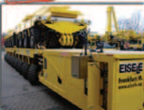
SPMT, Y.2009, 26 axle, turtable, driver- cabin, PPU Z350 and PPU Z100
