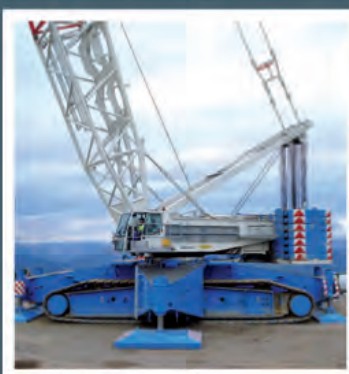
Demag CC2800, 600 ton capacity
