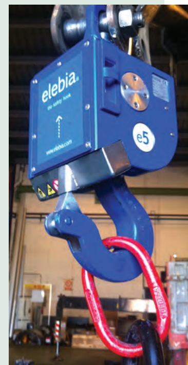
The second generation of Elebia auto-release hooks
