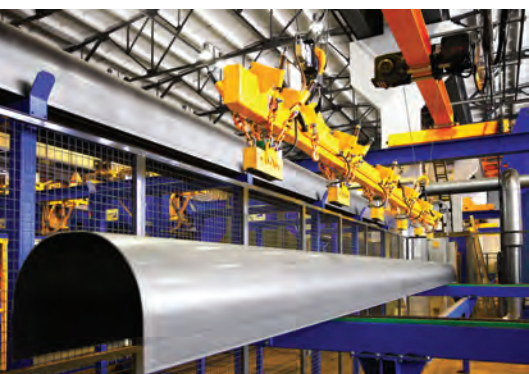
Avtokran is building U-section telescopic booms for its 16 to 80 tonne capacity truck crane range
