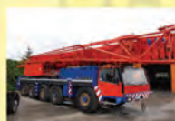
Liebherr LTM 1220-5.2 120 t YOM
