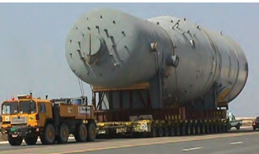
A pull type transport with prime mover and drawbar
