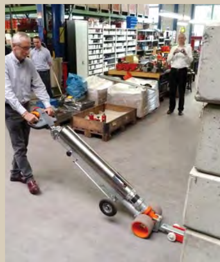
The PowerAttack can pull up to 55,000 pounds (25 tonnes)
