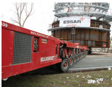
The self propelled modular transporter turning at the entrance to the Stanlow refinery
