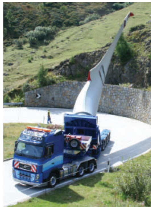
Transport of the first rotor blade: the team mastered the 15 m hairpin bend radius in 3 minutes
