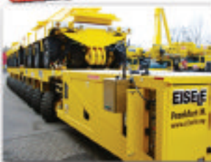
SPMT, Y. 2008, 26 axle, turntable, driver cabin, PPU Z350 and PPU Z100
