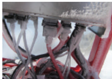
Ice build up on the slewing ring gear and on the electrical connectors
