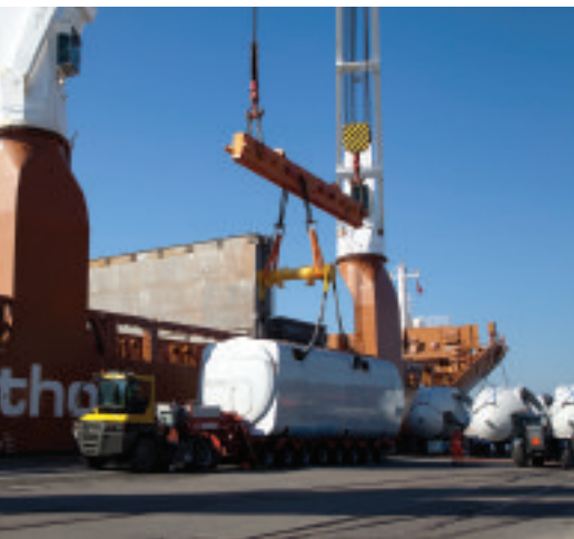
A Vestas nacelle is lowered into awaiting dockside transport
