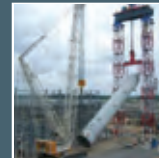
TEREX DEMAG CC2800-1, 600 ton capacity
