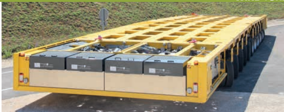
A self-propelled modular transporter – the Nicholas MHD G2 with hybrid drive – used at the new Alstom wind turbine manufacturing facility in St Nazaire, France
