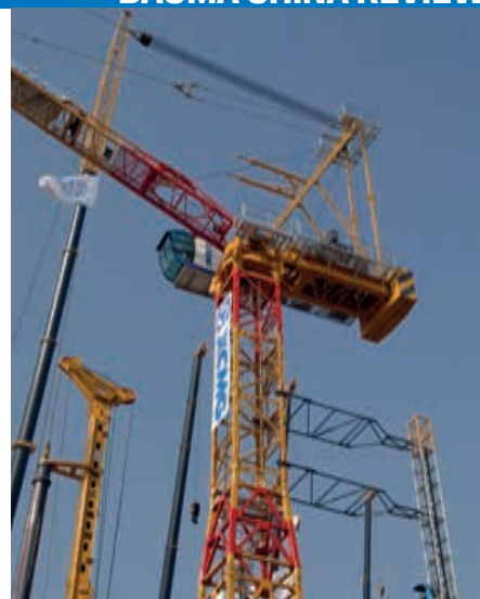
The 20 tonne capacity XAL6025-20 is described by manufacturer XCMG as a multi-functional dual purpose tower crane with a luffing and horizontal jib. XCMG says it is easy to switch modes between high capacity luffer and efficient horizontal jib tower crane
