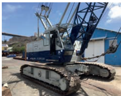
Kobelco 7065 Crawler Crane
