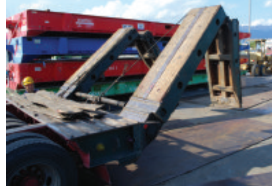
Lowering the ramps over the steel plates
