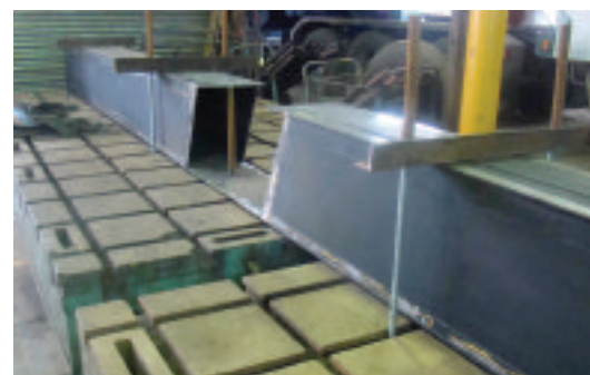
A tee slot bed at Crowland in the UK used for boom and other repairs
