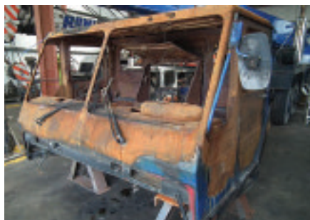
When a crane catches fire sufficient heat can be generated to damage the boom and other structural components
