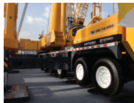
XCMG's XCT220 is a new 220 tonne capacity truck crane on leaf-sprung axles
