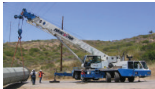
A Maxim Link-Belt HTC8670, which has 70 US tons (64 tonnes) capacity, replacing de-energised power poles in San Diego, USA
