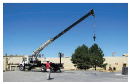
A 16 US ton (14.5 tonne) capacity Manitowoc National Crane NBT16 boom truck at work
