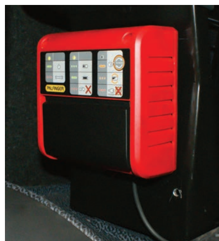
The battery charging station for the PALcom P7 radio remote control installed in a truck cab
