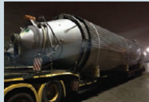
The 15 tonne silos measured 18 metres long, 3.6 m high and 3.3m wide
