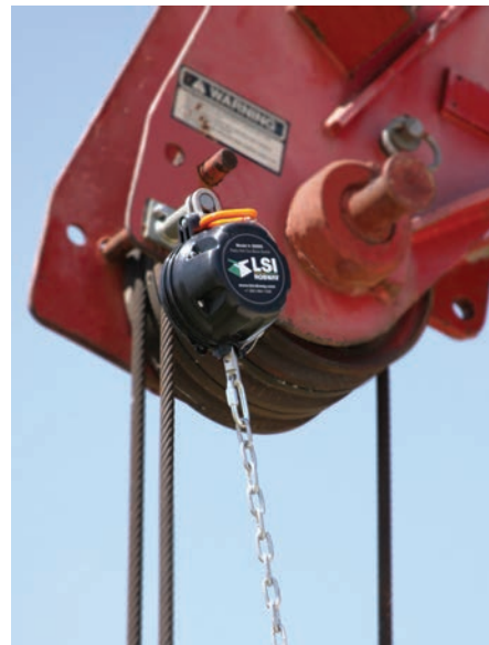
New from LSI-Robway is the GS085 anti-two block switch and line of wireless load cells to go below the hook
