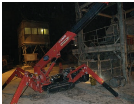
A Unic URW-095 mini crane from GGR Group works 182 metres underground at the Winsford Rock Salt Mine in Cheshire, UK
