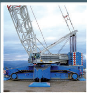
Demag CC2800, 600 ton capacity
