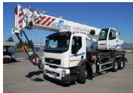
The MTK 35 has a lifting capacity of 35 tonnes and is on three axle truck chassis
