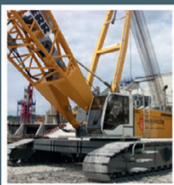
LIEBHERR LR1300, 300 ton capacity
