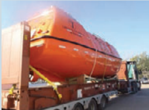
The lifeboats were transported to Piraeus Port on 12 metre long flat racks
