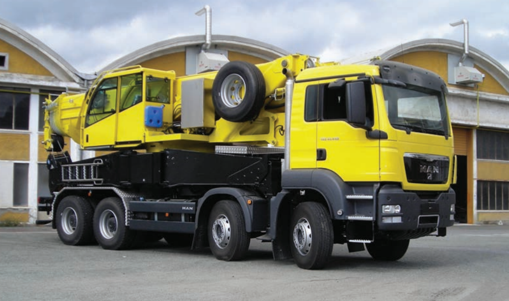
The Ormig 104AC has a 100 tonne lifting capacity, an 8-section telescopic boom and can travel on most motorways and roads without transit permits
