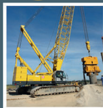
Kobelco CKE2500, 250 ton capacity
