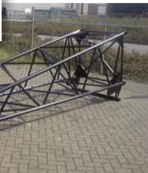
Before and after. Rusch Kraantechnik in the Netherlands repairs a twisted lattice boom section
