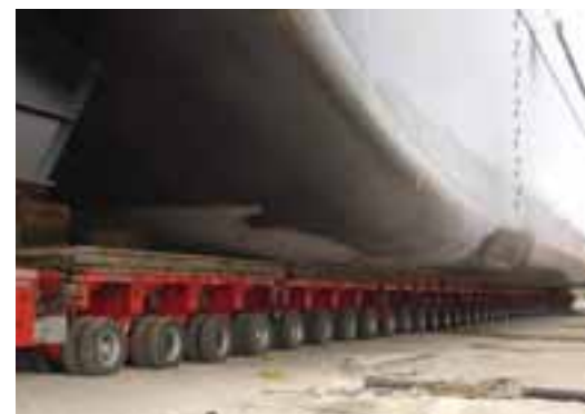
Berard Transportation, Inc. used a mixture of its mechanically and electronically steered Goldhofer modular trailers
