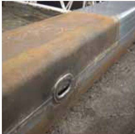
Dented boom section repaired by Rusch Kraantechnik
