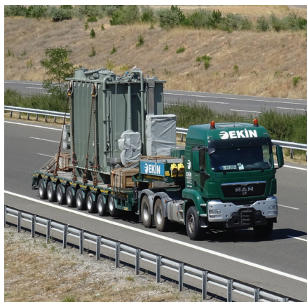
The transformer was 6.6 metres long, 2.45 m wide and 4.0 m high and weighed 86 tonnes. It was transported through Turkey to Hakkari
