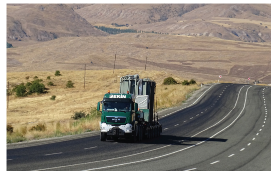
The transformer was 6.6 metres long, 2.45 m wide and 4.0 m high and weighed 86 tonnes. It was transported through Turkey to Hakkari
