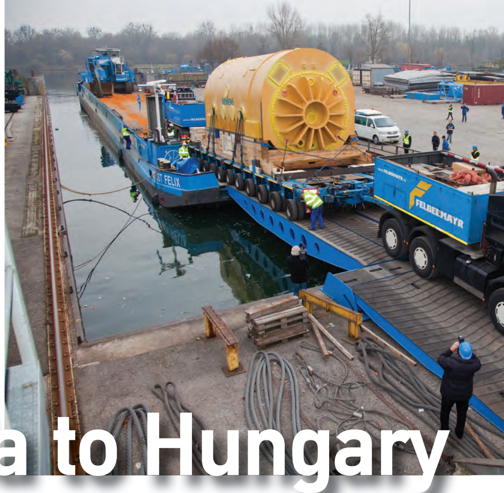
A 1.5 coupled 12-axle heavy low-loader trailer moves the generator onto the Horst Felix
