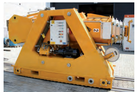
The SBL1100 foldable boom and mast section is ideal for low-height clearances
