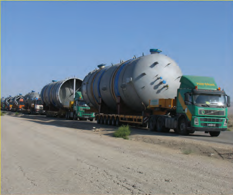
Transportation of total 66 units oversize and heavy equipments max. 35m. length, 7,6m. width, 8,2m. height and 270 tons weight from Turkmenbashi Port to Yoleten Turkmenistan total 1250 km. distance.
