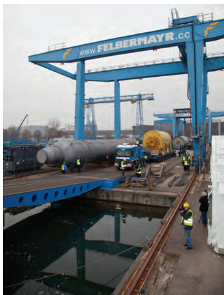
A 1.5 coupled 12-axle heavy low-loader trailer moves the generator onto the Horst Felix
