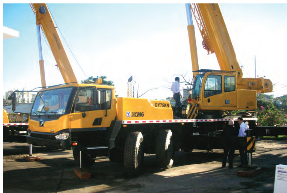
XCMG has developed its QY75KN telescopic crane for the Brazilian market. It is a truck crane that includes features usually found on an all terrain crane
