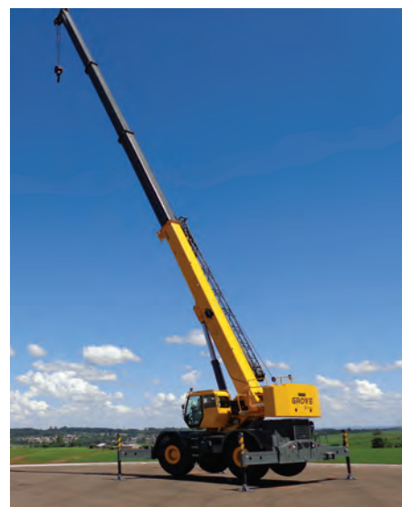
A 60 US ton capacity Grove RT765E-2 rough terrain crane built at Manitowoc's Passo Fundo factory in Brazil
