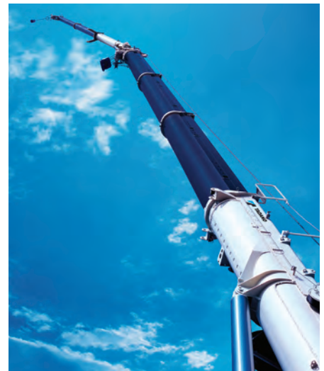
A Tadano ATF 220G-5 fitted with a hydraulic telescoping luffing jib
