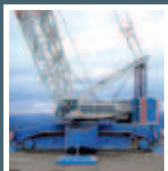
Demag CC2800, 600 ton capacity
