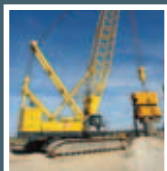
Kobelco CKE2500, 250 ton capacity
