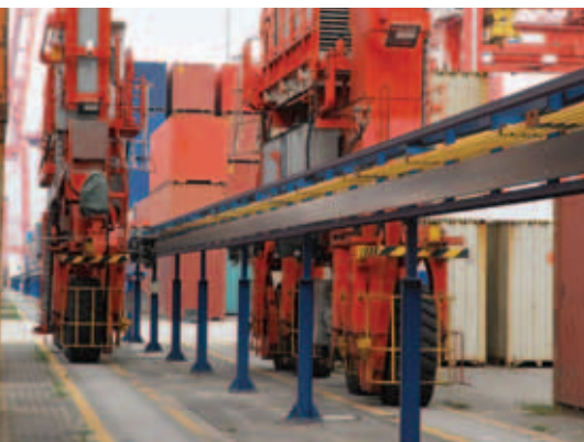
Conductix-Wampfler will convert RTGs in the Turkish port of Yilport with its Drive-In system
