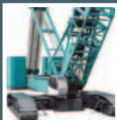
Kobelco SL6000, 600 ton capacity
