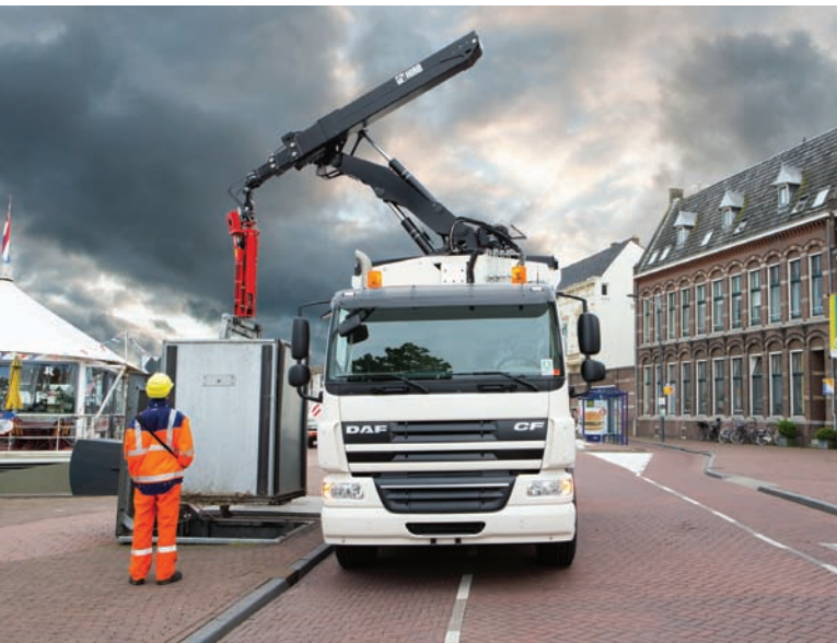
The Hiab S-HiPro 130 crane is designed for mounting on top of a vehicle
