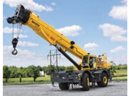
New from Manitowoc is the 90 tonne capacity GRT8100 rough terrain crane
