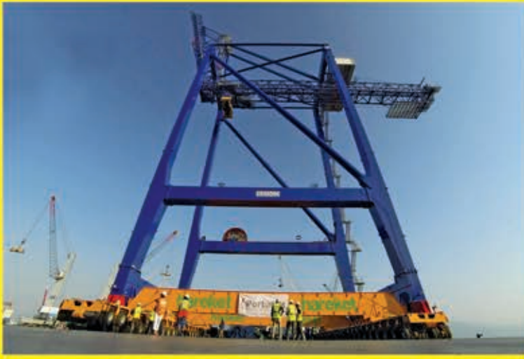
Transportation of 1256 tons Liebherr Port Crane with 2 pcs. 24 axles 2 file Goldhofer PST/SL-E trailer.
