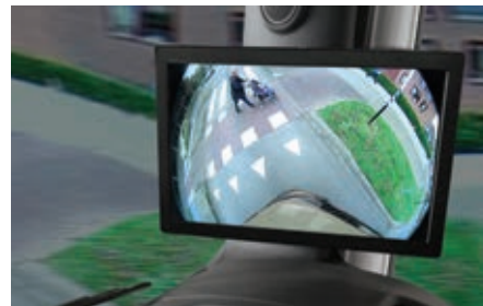
Orlaco Corner Eye camera offers a 270 degree field of view
