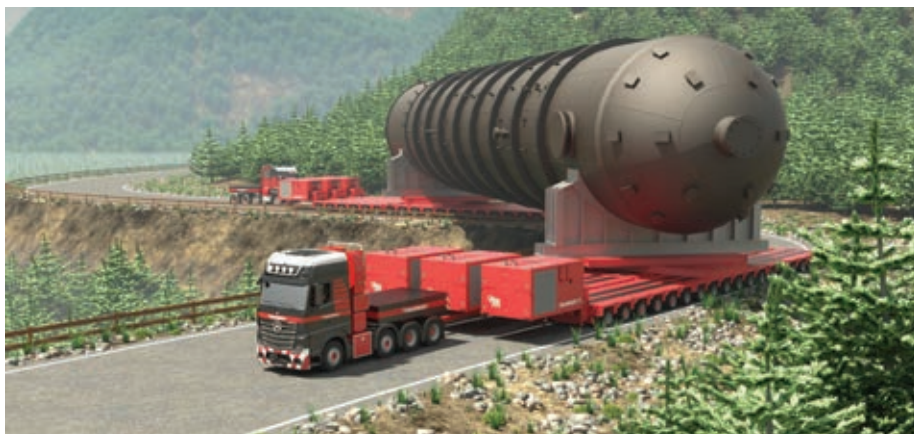
Scheuerle and Mammoet have developed the 1,000 hp Trailer Power Assist (TPA) system
