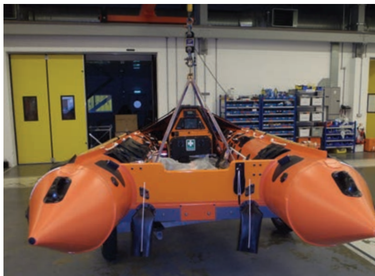
The RNLI sea rescue service in the UK uses Straightpoint load cell while lifting D class, Atlantic 85 and other lifeboats
