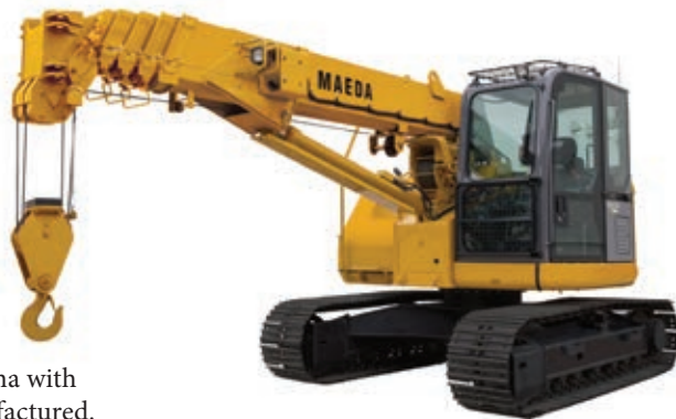
Maeda has updated its CC1485 crawler crane
