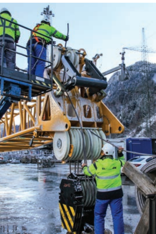
Left: Liebherr and Teufelberger have jointly developed a synthetic fibre hoist rope for cranes that is being tested. Above: Scania R 730 LA
