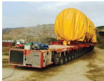
Transport was on 24 axle lines of self propelled modular transporter (SPMT)
