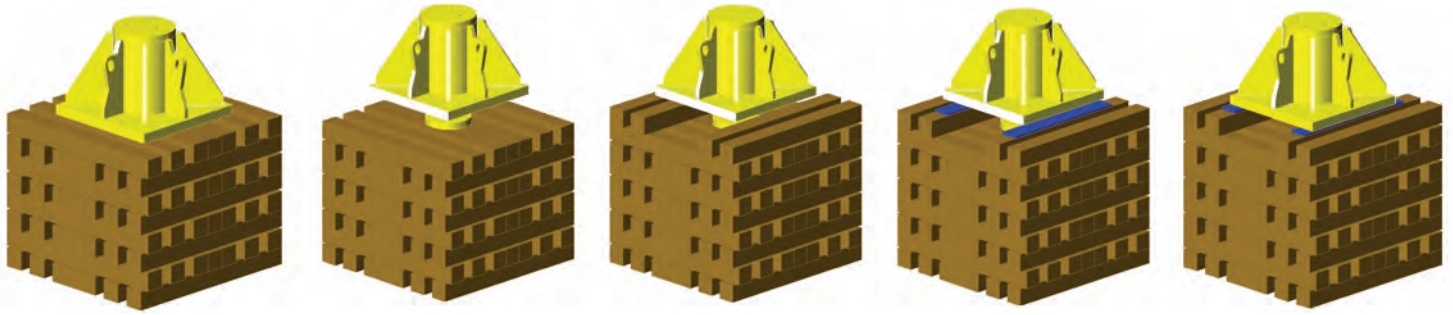
FIGURE 1 Using hydraulic jacks to raise a load to a significant height is a laborious process
