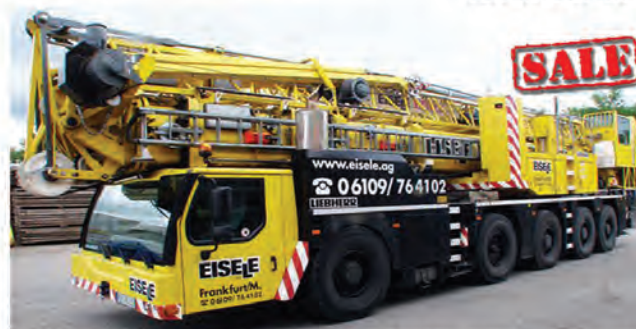
Liebherr MK 110, year 07/2006, maximum capacity 8 t/14 m, maximum radius 52 m/1,8 t
