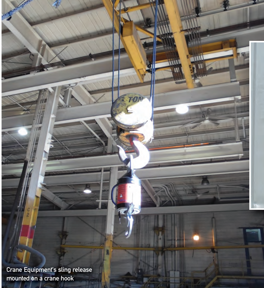
Crane Equipment's Baby Babe and Babe remote controlled sling releases
