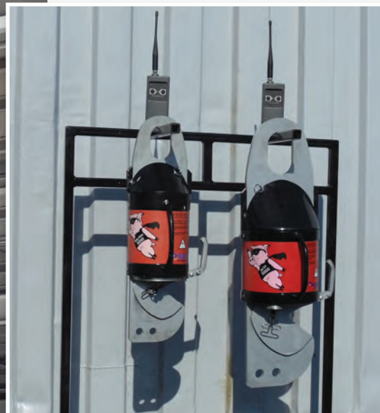
Crane Equipment's Baby Babe and Babe remote controlled sling releases
