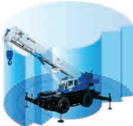
LMI technology on Tadano rough terrain cranes automatically detects the extension width of the outriggers
