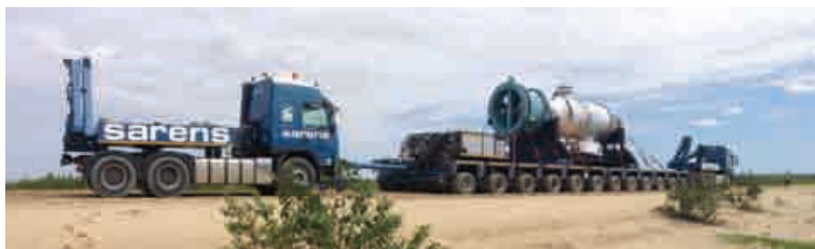
Transdata use SPMT to transport a pipe rack internal haulage at a petrochemical facility in Rio de Janeiro, Brazil
