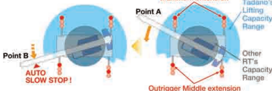
Tadano's LMI technology monitors continuously to maintain a safe operation
