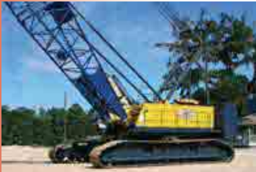
470 is the Kobelco 7150 (165-ton #470) Two machines in stock
