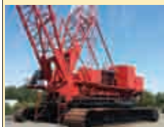
MANITOWOC Model 7000 350/800 ton cap. Crawler Crane
