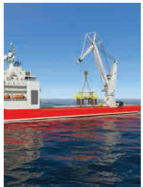
Huisman’s 900 tonne rope luffing knuckle boom crane
