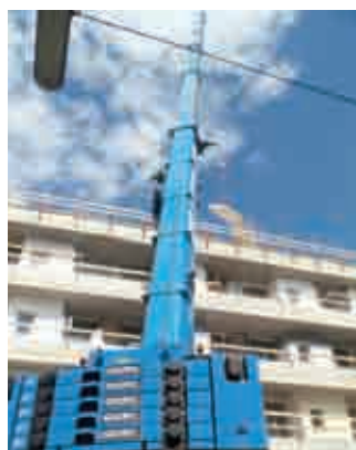
The Grove GMK6300L has an 80 metre boom and offers a lifting height of nearly 120 m
