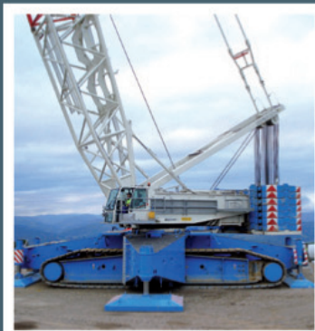
Demag CC2800, 600 ton capacity
