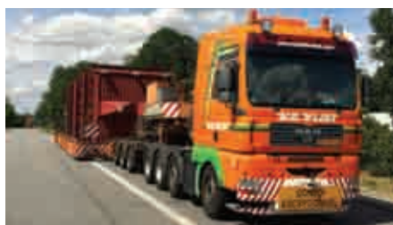
The boiler was loaded onto an 8-axle semi low loader trailer for the final section to Épinal
