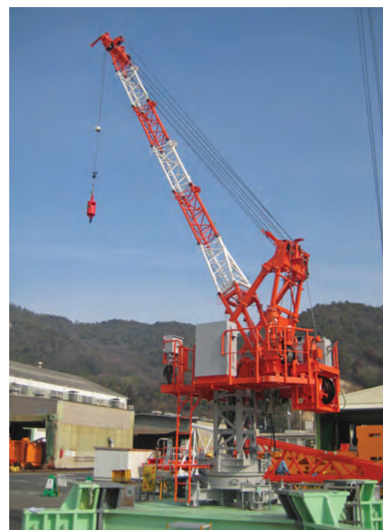
The small JCC-V10SK dismantling crane on the test ground in Yasuura. Note the inserted pin-connected tower raising the upper crane above the slewing unit for extra under hook height
