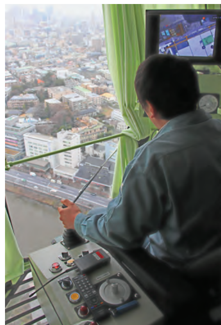
Inside the cabin of the JCC-V700 is the large monitor for the hook camera on the right side
