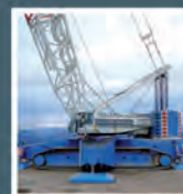
Demag CC2800, 600 ton capacity
