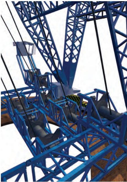
The winches in their frames form part of the CRC crane structure
