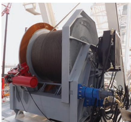
LEFT: Disk brake on the Yongmao STL1460C hoisting winch
