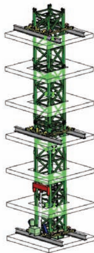
Fixing the tie-in beams using the work platform
