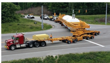
Crane Rental Corp dual lane trailer making a 90 degree turn
