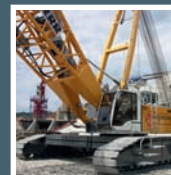
LIEBHERR LR1300, 300 ton capacity
