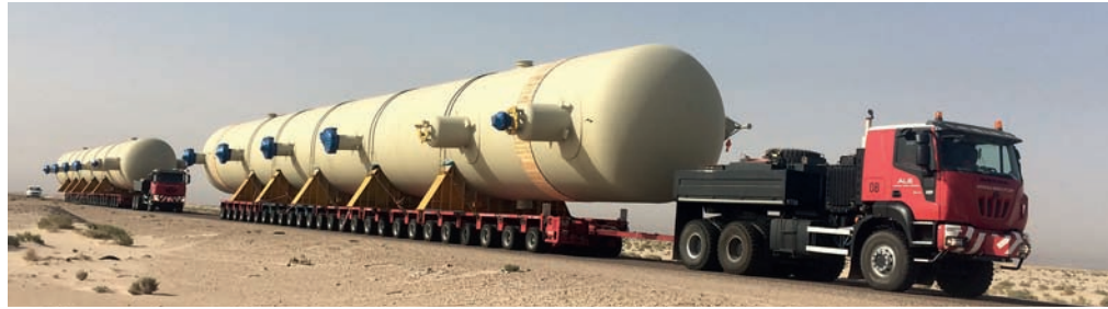
The tanks were moved using 2 x 24 axle lines of conventional trailers
