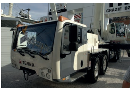
Terex's new 100 tonne T110 truck crane unveiled at the ConExpo show in Las Vegas in March 2017. Unlike other US-market truck cranes, the Terex T110 has a two-seat driver cabin for moving between jobs
