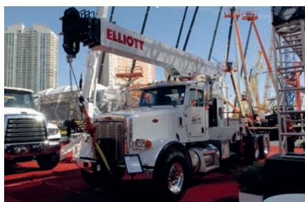
Elliott's model 1800 straight boom loader crane mounted behind the cab and ahead of the fifth wheel coupling on a three-axle tractor
