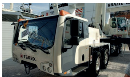
An AT-style double cab for the driver is a distinctive feature of the new Terex T 110, a 100 tonne capacity truck crane
