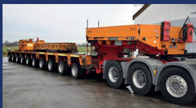
Goldhofer THP-L 4+6 excavator + vesselbridge
