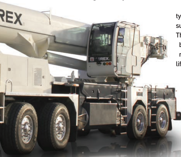
Terex's new 100 tonne T110 truck crane unveiled at the ConExpo show in Las Vegas in March 2017. Unlike other US-market truck cranes, the Terex T110 has a two-seat driver cabin for moving between jobs
