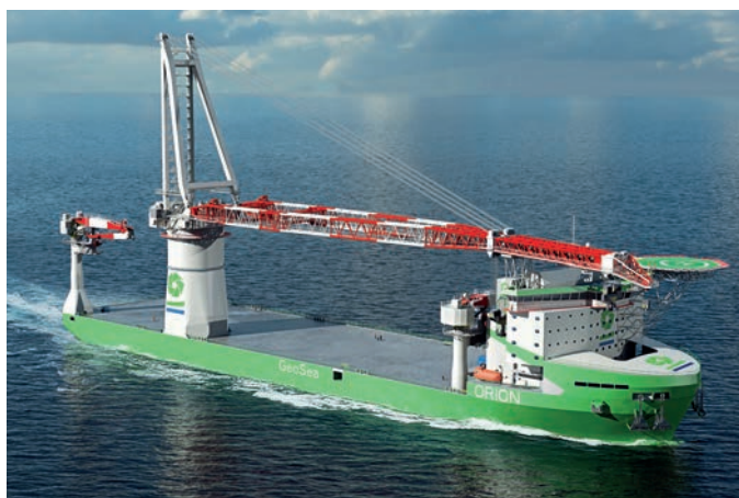
How the new 3,000 tonne capacity Liebherr HLC 295000 heavy lift offshore crane will look mounted on Deme's next generation offshore installation vessel, Orion
