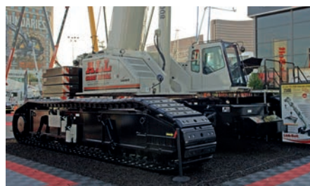
Link-Belt's new range-topping 250 tonne capacity TCC-2500 telescopic boom crawler crane was an imposing sight. This one was destined for leading US rental house All Crane Rental
