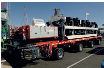
Scheuerle's dual lane Highway Giant with Power Booster module can be folded and loaded up on a trailer for empty return legs
