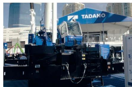
Tadano's new 120 US ton (110 tonne) capacity rough terrain on two axles, the GR-1200XL. It has a 56 metre boom and up to 17.7 metres of extensions can be added. Its (8.65 m long)
