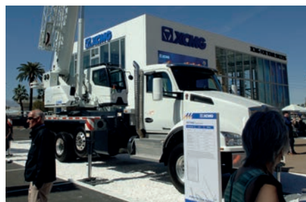
XCMG's 40 US ton (36 tonne) capacity model XCT40U truck-mounted crane has a 43 m, five section boom. Its maximum length is 59.6 m
