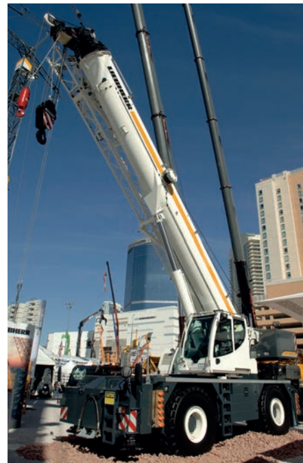
Liebherr's new LRT 1090-2.1 rough terrain crane. It is the 90 tonne capacity model, smaller brother to the 100 tonne LRT 1100-2.1. Both were on display and generated strong interest, especially with their Cummins engines
