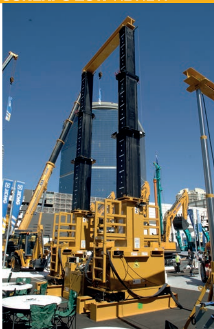
Lift Systems was out in force with its hydraulic telescopic heavy lifting gantry systems
