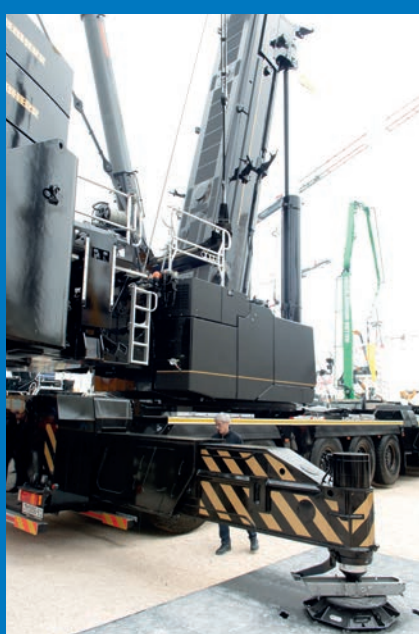
The first unit of Liebherr's new LTM 1650-8.1 wheeled mobile telescopic crane was handed over to German crane rental company Riga Mainz. Capacity is 700 tonnes and there are 54 and 80 metre boom options
