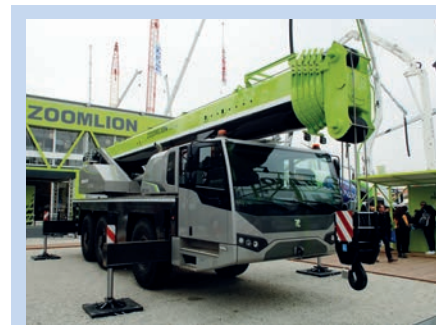
The ATC960 is a 60 tonne capacity all terrain designed and produced in Italy, said manufacturer Zoomlion. It has a 51 metre, six-section boom and a three-axle carrier
