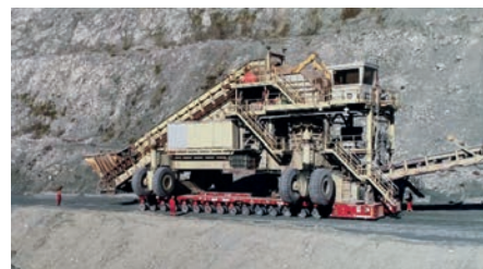
Transport of the 690 tonne rock crusher on SPMT
