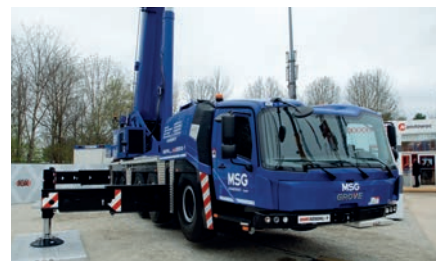
Above: The new Grove GMK5250XL-1 boasts the longest boom on five axles, said manufacturer Manitowoc. The 250 tonne capacity all terrain has a 78.5 metre boom
