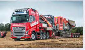
Limehillock Quarries' Volvo FH16-750 being used with a four-axle rear-steer Nooteboom trailer
