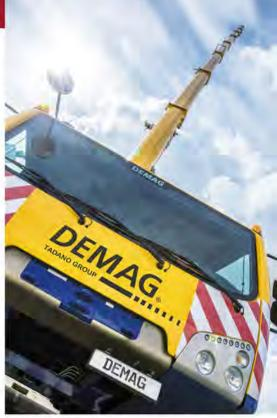
A 220 tonne capacity Tadano Demag AC 220-5 all terrain crane in Tadano Demag colours
