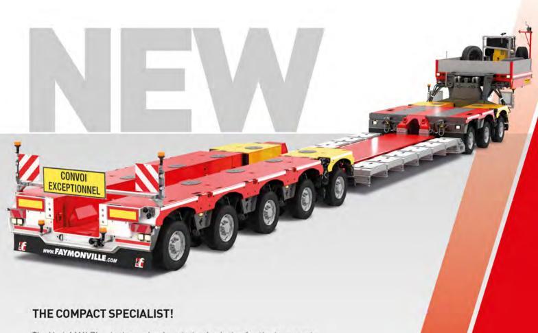
The VarioMAX Plus is the payload-optimised solution for the **transport** of heavy construction machinery, mobile conveying and crushing systems as well as **transformers**. The strengths of the VarioMAX Plus low bed trailer are its high payload capacity, modular versatility and agile handling.
