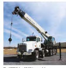
The NBT60L is a 60 US ton model with 46 metres of main boom
