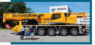
boom in its tonnage class, the manufacturer said. It has 151 feet (46 metres) of main boom and a maximum main boom height of 161 feet (49 metres). It can have a 36 foot (11 metre) off-settable lattice jib that extends reach to a 196 foot (59.7 metre) maximum tip height.
