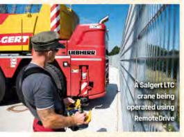
German crane rental house Salgert has taken delivery of two new Liebherr LTC 1050-3.1 compact cranes. These are the first cranes to have RemoteDrive – a feature that allows the crane to be operated via remote control from outside the cab. This is particularly advantageous for crane operators working on congested sites, Liebherr said, as it enables the operator to obtain a better view of their work.
