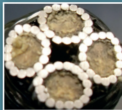
FIGURE 1: From left to right; a) Cross-sectional drawing of the 4-strand hybrid rope b) Cross-sectional cut-view of the 4-strand hybrid rope
