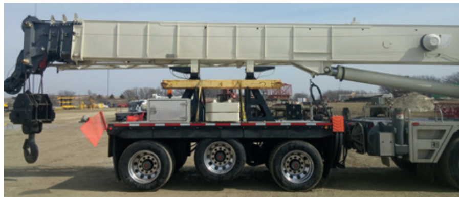
HMR dolly models are available with single, split or tilting tower options. Three axle dollies are available with an optional lift axle, and three or four axle dollies are available with caster axles.
