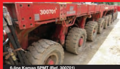
6-line Kamag SPMT (Ref. 300701)
