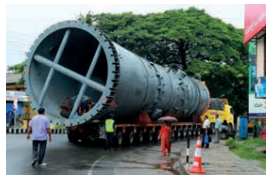
Shipment belonging to G R Engineering being shifted by Resham Singh's Goldhofer multi-axle trailers through the narrow roads of Kochi
