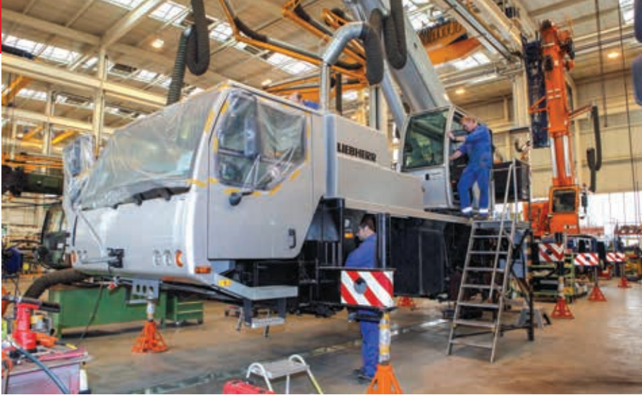
Liebherr staff working on the repair and refurbishment of an all terrain crane
