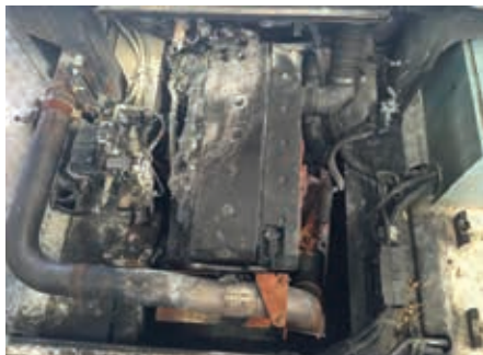
Crowland Cranes repaired the damage from an engine fire on a Tadano ATF 40G all terrain crane
