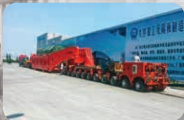
Auxiliary Drive Hydraulic Modular Transporter+Girder Bridge
