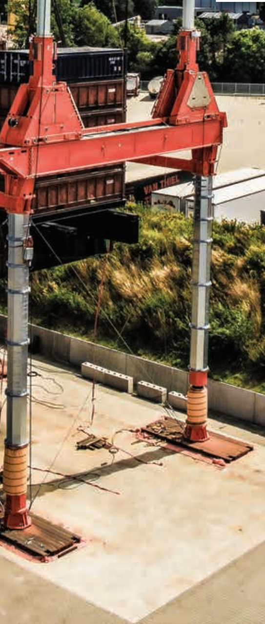
Grand proportions: 450 tonnes capacity and 15 metres lift height
