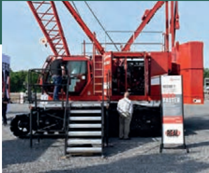
Dubbed by Manitowoc as “the only 100-ton crawler crane proudly made in America” the MLC100-1 was designed for quick and simple erection.
