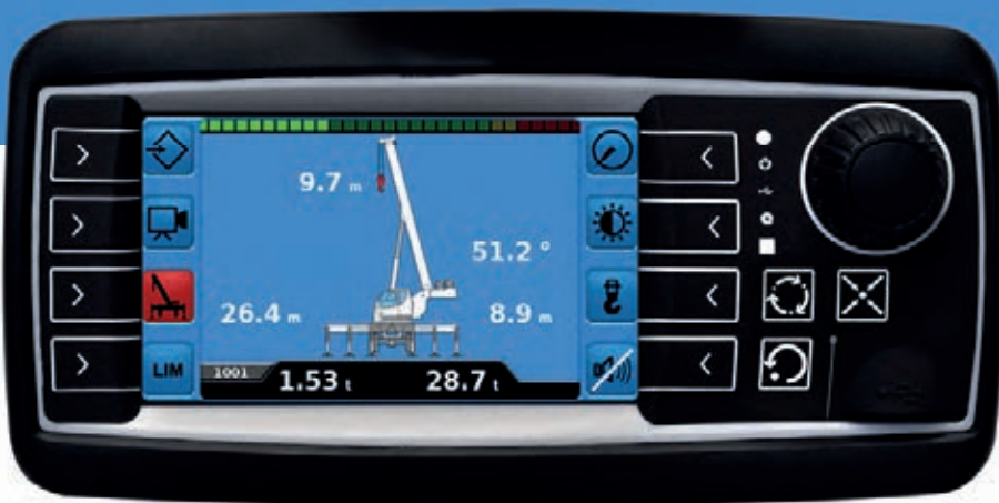
The qSCALE Ix LMI provides a display of the crane's current load and geometric information.
