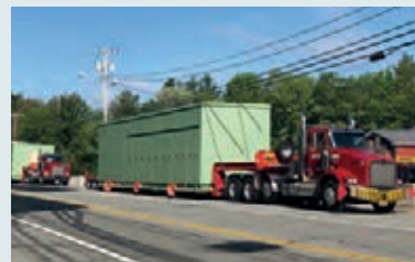
The 3-axle trailers on air suspension are rated for 100,000 pounds technical capacity.
