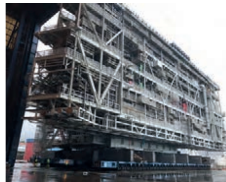
Sarens used 432 lines of Kamag K24 SPMT
