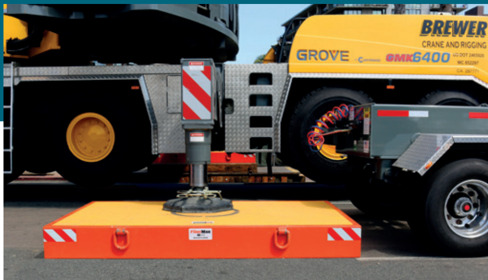
Brewer Crane and Rigging of Lakeside, CA reports it can move DICA's FiberMax crane pads up to 75 percent faster than heavier wood mats or steel plates.
