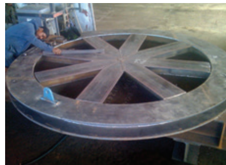
Left: Hydraulic cylinder for turning the turntable with its load; Above: the engine on the turntable Right: The turntable ring in fabrication
