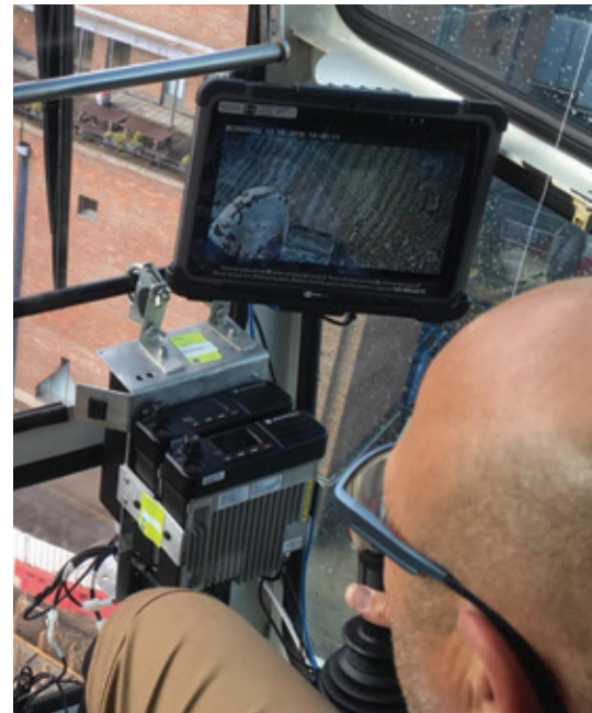
The BlokCam monitor inside the crane's cab gives the operator an unobstructed view
