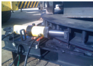
Left: Hydraulic cylinder for turning the turntable with its load; Above: the engine on the turntable Right: The turntable ring in fabrication
