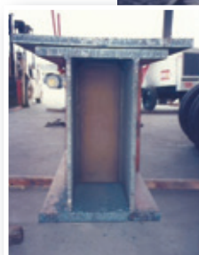
Above: Vertical webs added to further stiffen the box beam
