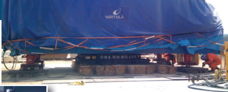
Left: Hydraulic cylinder for turning the turntable with its load; Above: the engine on the turntable Right: The turntable ring in fabrication
