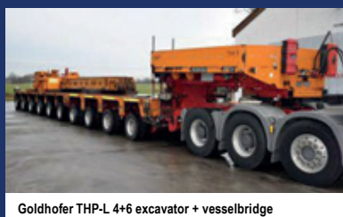
Goldhofer THP-L 4+6 excavator + vesselbridge
