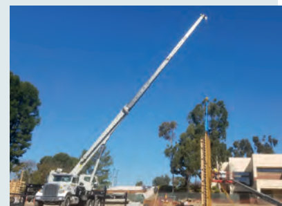
Crainco's NTC55 has a 55 ton capacity and a 128-foot reach.
