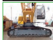
90 t Liebherr HS 853 HD Boom 32 Metre
