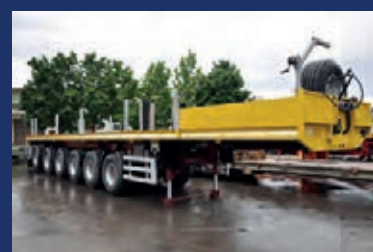
HRD 6 axles ballast trailer
