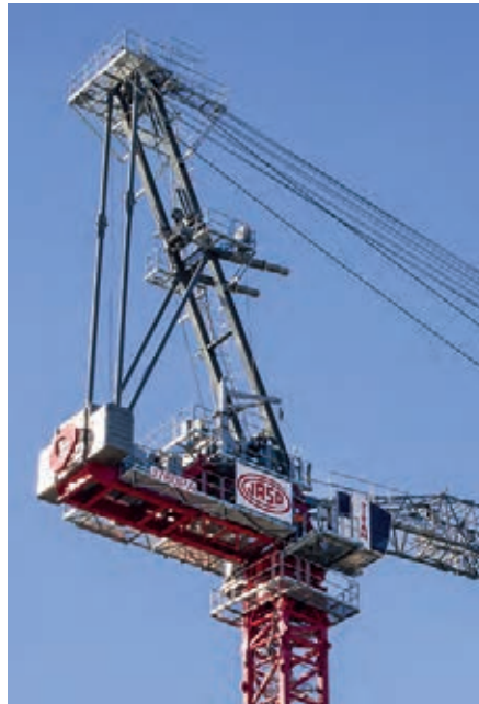
Double deck counterjib of the all new Jaso J780PA with one hoisting motor on top positioned parallel to the drum to save space
