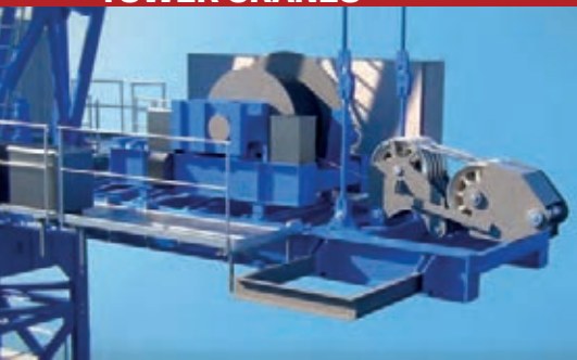
Placing the hoisting winch at the front leaves plenty of access room at the counter jib with the pre-reeved luffing rope arrangement
