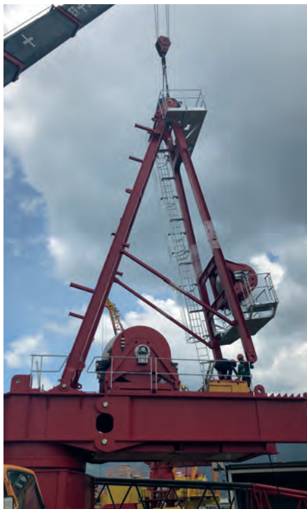
After minor modifications of the upper crane design, reducing the number of falls and replacing the boom nose with a standard jib end section for two fall operation, the Krøll K1650L becomes a versatile heavy lifter for precast concrete construction in Singapore
