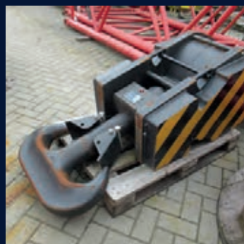
Used hookblock 5-sheave Grove GMK6300L yom 2014
