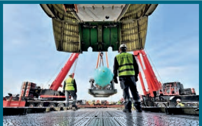
Heavy lift and transport specialist Mammoet loaded four 140 tonne reformed-gas waste heat boilers onto the world's largest cargo plane – the Antonov AN-225 Myrna – at the Leipzig/Halle Airport in Germany.
