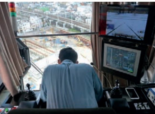
An inside view of the Kitagawa JCL1000NK ergonomic crane driver cabin with a large hook camera monitor and a multi-functional touchscreen
