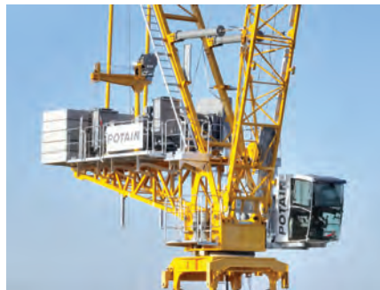
The Potain MR 309 features a jib that can be mounted horizontally in one or two parts to minimize space requirements during erection.
