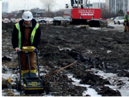
Geophysical methods collect data over wide swaths and broadly offer a depiction of subsurface conditions across the site. Analysis of this data allows for the identification of subsurface voids and areas of unconsolidated soils, with their positions and extents being estimated.
