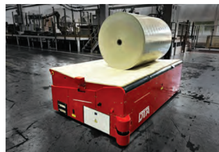
Enerpac's self-propelled electric transporter.
