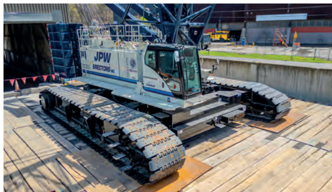
The 348 Series 2 used 200 feet of luffing boom and 160 feet of luffing jib to lift the flues to the top of the stack and lower the old sections for transport.
