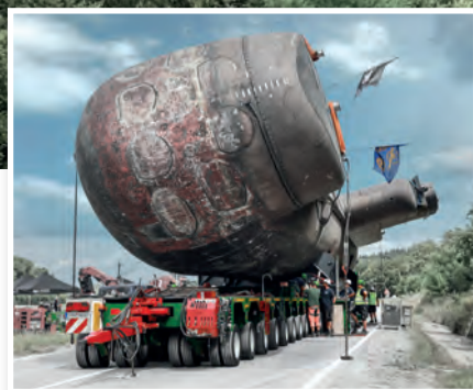
The world's first rotation of a submarine on a modular platform trailer.
